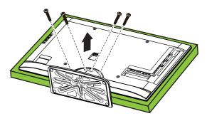
**3** Secure the stand cover to the back of the TV screen using the four screws you just removed.
